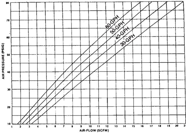
Air Flow vs. Air Pressure (60 GPH Nozzle)
