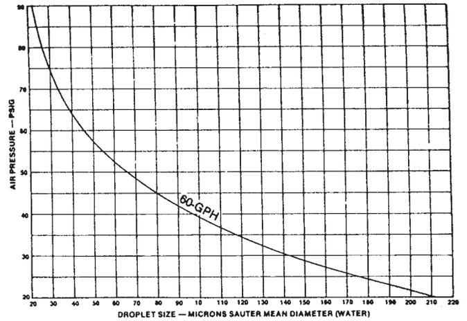
Droplet Size vs. Air Pressure (60 GPH Nozzle)
