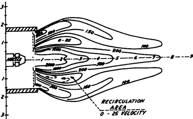
Figure 3. Pattern produced by a flame retention burner.
