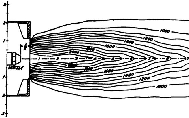
Figure 2. Typical air pattern for a convention burner with a static disc and cast-iron end Cone.
