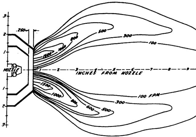
Figure 1. Definitely hollow air pattern for one type of burner. This pattern is from a Shell Head burner.
